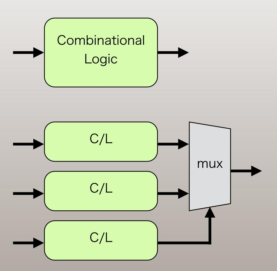
Condition affects on # inputs of MUX and # MUX stages
